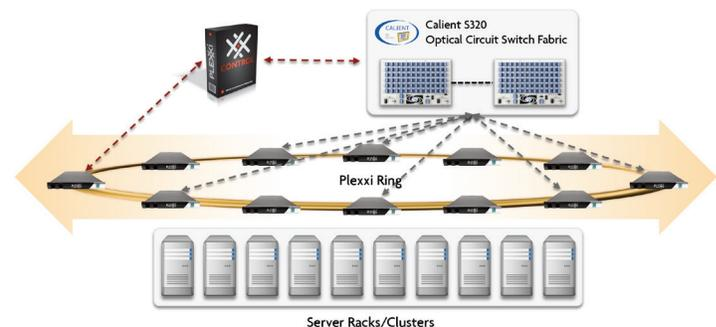
The key to the hybrid packet-optical architecture is that the packet and optical elements must co-exist and be coordinated by higher-level management layers. In SDN terms, this coordination happens through a controller. In the Plexxi-CALIENT integration, Plexxi Control serves this role.
