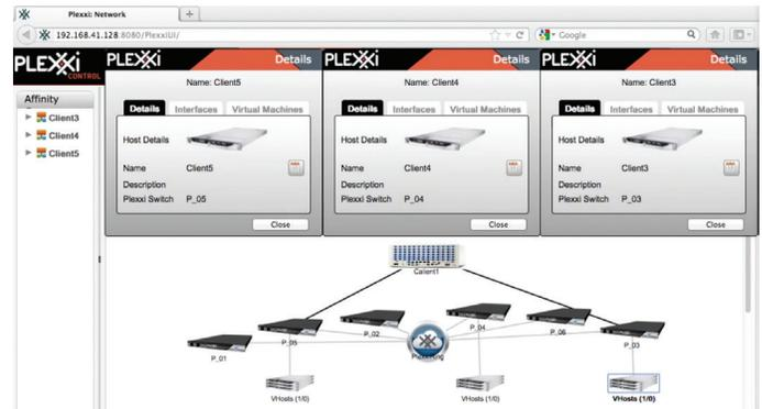
The above screenshot shows an affinity between hosts connected to switches 3 and 5. When traffic between them enters the Plexxi network, the affinity isolates that traffic on the links to the CALIENT S320.
